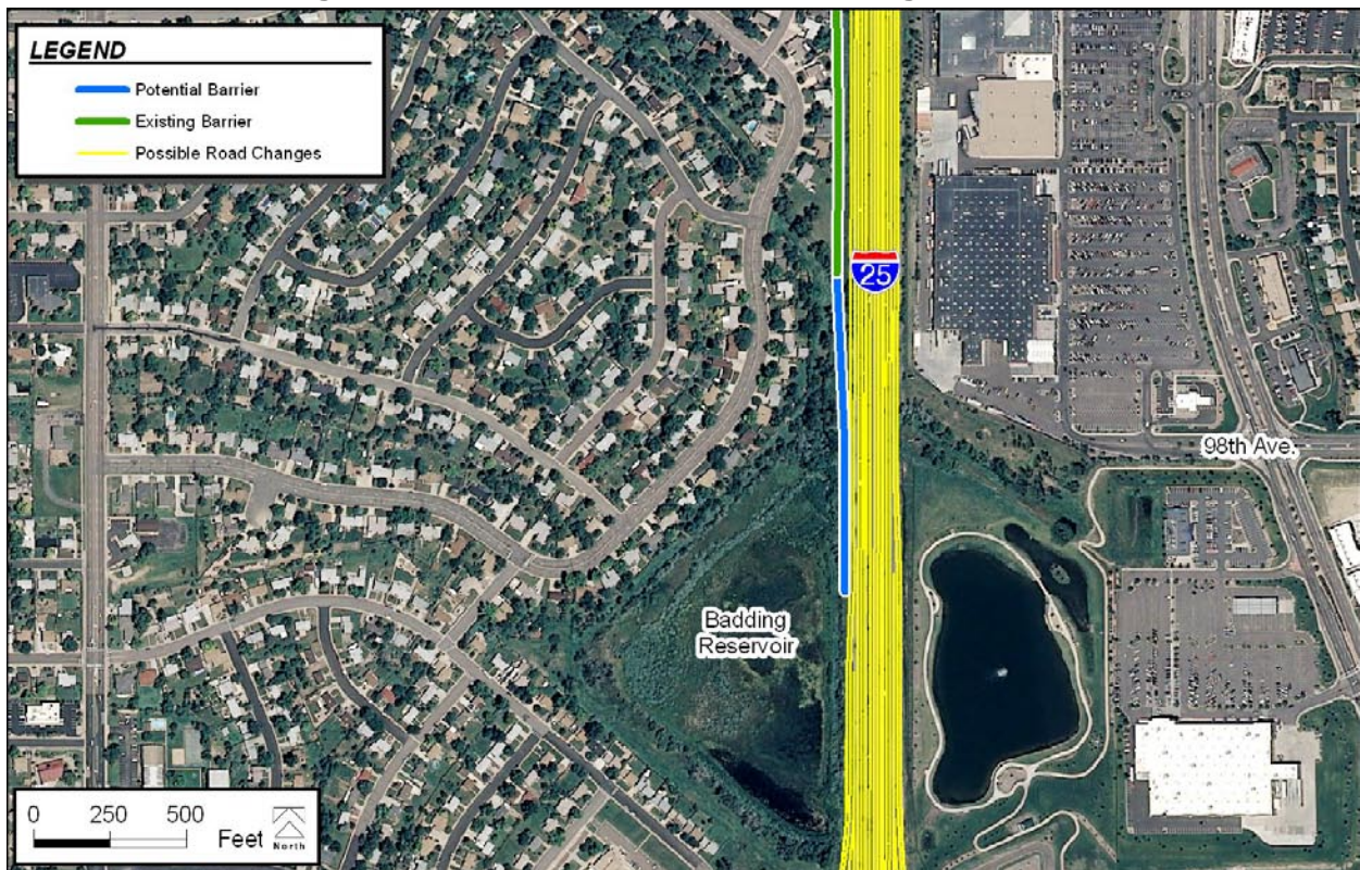
Figure B-14. Barrier Extension at Badding Reservoir
